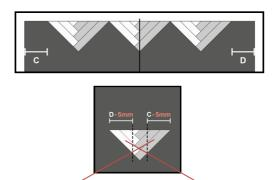
5. The last triangle is used to fill the free space on the left and right. Measure both free spaces and bear in mind the expansion gap of at least 5 mm. Use the left-hand part of the triangle at the right side and the right-hand part of the triangle at the left side
