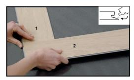
2. **Next, take an R panel** (n°2) and position the long side of the R panel at an angle of 90° against the short side of the previously installed L panel (n°1). Make sure that the grooves of the two panels are always in a straight line, and slotted firmly together.
