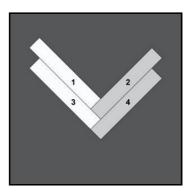
3. Place a second L panel (n°3) with the long side in the long side of the previously installed L panel (n°1) and into the short side of the first installed R panel (n°2), according to the tongue-and-groove system. Make sure that the groove of the short side of the second L-panel (n°3) forms 1 straight line with the groove side (on the long side) of the first R-panel (n°2).
